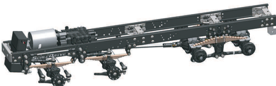
8x4 chassis with ScaleDRIVE components: version 2
